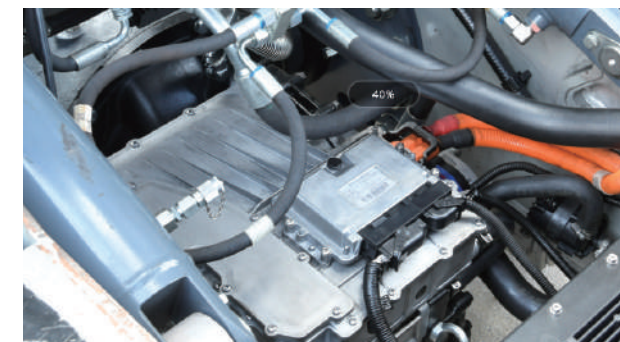
The integrated power system reduces the wiring harness which greatly reduces the loss of electric energy transmission. And the levels of parts and control modules are clear and convenient for maintenance;
